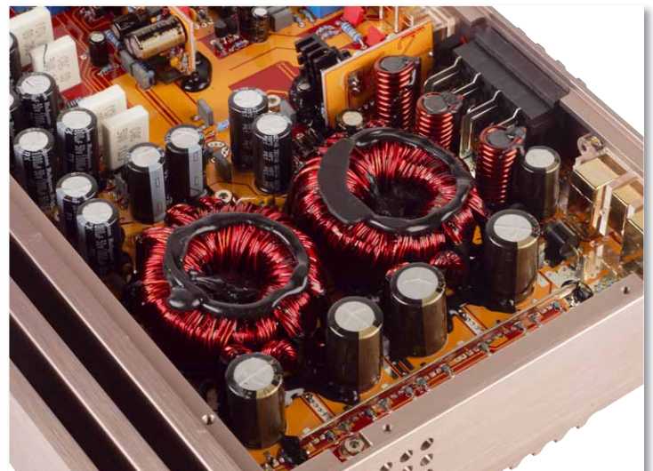
The GZUA 6SQ houses two power supplies, one for the small and one for the large channels
